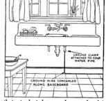
of the ground wire. Scrape the bare wire until it is bright, and attach this bared end to the terminal on the ground clamp. Cover the clamp with vaseline to prevent corrosion of the pipe.
